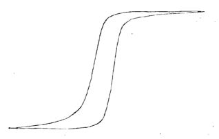
a finite area, indicating the dissipation of a finite quantity of energy proportional to the area of the curve, and this dissipated energy will appear as heat.
