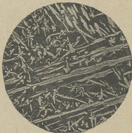
Fig. 14. — Cu = 56,5; Zn = 43,5. Laiton =  $\alpha + \beta$ .
